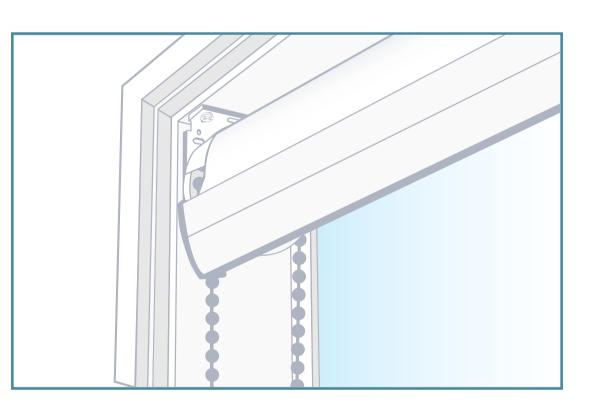
Gently slot the chain end into the chain drive bracket.
