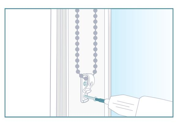
Screw the p clip onto your frame, using your cordless drill with the Phillips head drill bit. Remember that attaching to a wooden frame or wall studs is best, otherwise do your homework.
