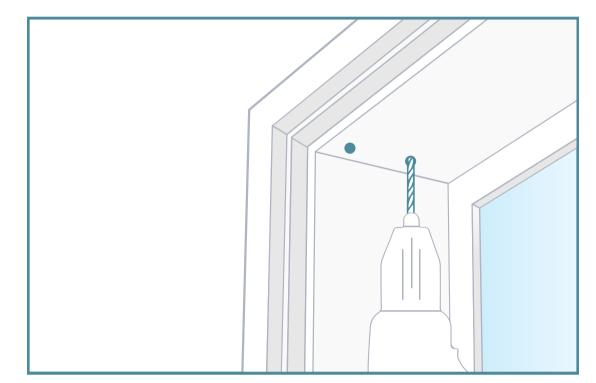
Using your cordless drill with the 3 mm drill bit, predrill 2 holes where you marked the two pencil dots.
