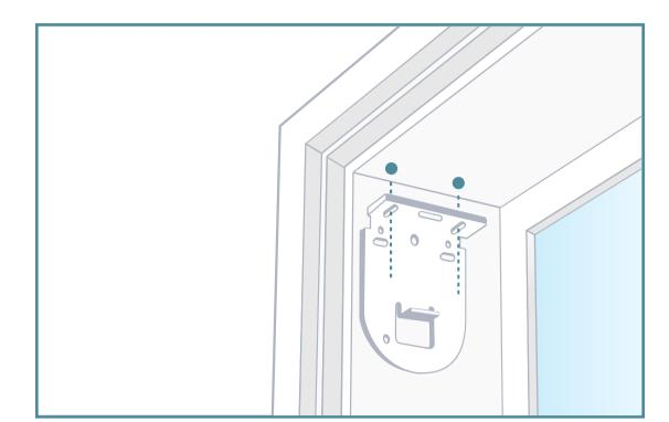
Take your pencil and both brackets. Lift each bracket up into position and mark two level dots where the screws will attach the bracket to the frame.
