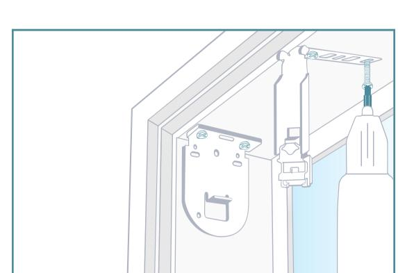
If you have a pelmet, pre-drill 2 holes for each pelmet sprung bracket, where you marked the pencil dots. Secure your pelmet sprung brackets with the screws in your custom kit, using your cordless drill with the Phillips head drill bit.
