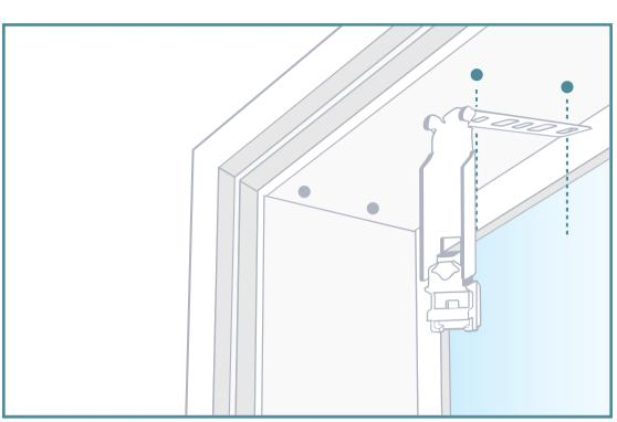
If you have a pelmet, take your two pelmet sprung brackets. Place each bracket on the underside of your frame at the top, a little way out from each blind bracket. Line up the face of the bracket with the front edge of your frame. Mark two dots where the screws will attach the bracket to the frame.
