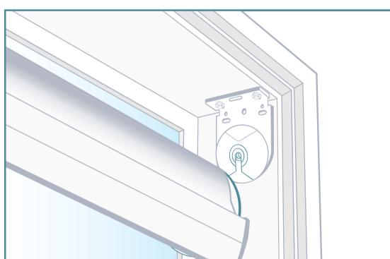
Then slot the pin end into the pin end bracket, until you hear a click.
