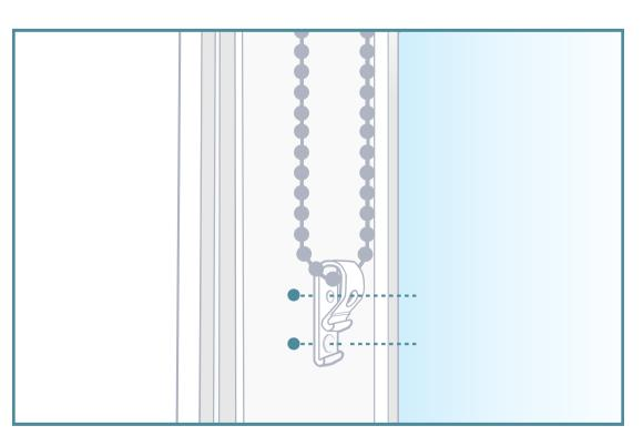
Click the p clip onto the bottom of the chain loop, then hold it into position and mark a dot where the screw will attach the p clip to the frame. Remember the chain should hang down with minimal tension.
