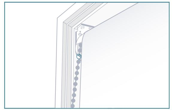
Use the ball stopper to adjust precisely where the blind rolls down to. Roll it down until you're happy with where it finishes, then grab your ball stopper and click it into the very top of the chain. This will help maximise the life of your blinds by taking some
