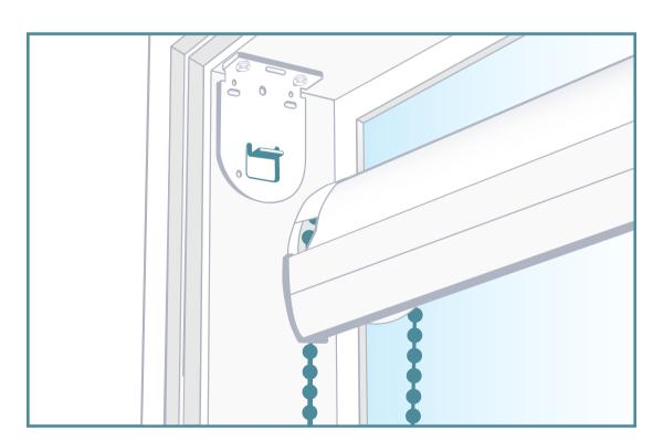
Pick up your roller blind and make sure your chain is on the same side as your chain bracket. Check that the hood over the chain is at 12 o'clock and the ACMEDA logo is at 6 o'clock.
