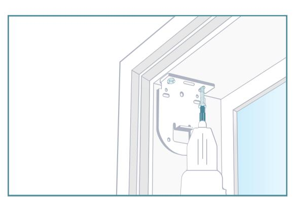
Pick up the chain drive bracket and position it on the side of the frame where your chain will sit. The holes in the bracket should be directly over the two holes you just drilled. Secure the bracket with the screws in your custom kit, using your cordless drill with the Phillips head drill bit.
