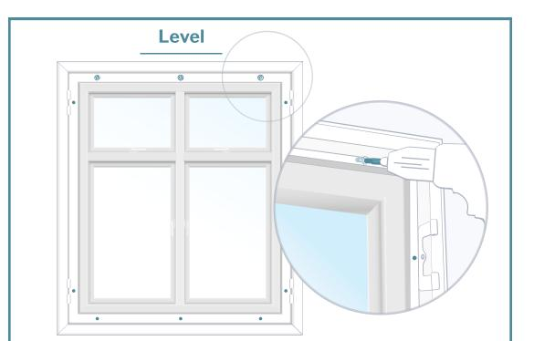
Wiggle the frame until you get it looking level across the top. You can rest a spirit level on top of the frame while you do this.
