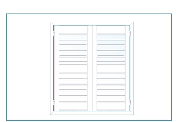
Check for a thin, even gap between each side of your shutter frame and your shutter panels.
