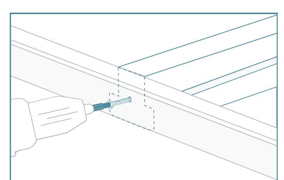
If you have T posts, screw them onto your shutter frame using your cordless drill and the long black screws in your custom kit. There are pre drilled holes on your shutter frame, to show where you'll attach the T posts. The top of your T post will be labelled t, and the bottom b.
