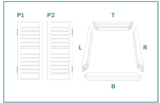
We label sections of your frame and your panels, which will help you to match up the right panels and hinges later. Lay out the shutter panels the right way up and in order from left to right.
