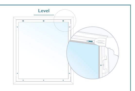
Wiggle the frame until you get it looking level across the top. You can rest a spirit level on top of the frame while you do this.
