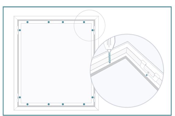
Turn over your shutter frame and lay it back down. Using your cordless drill with the 3 mm drill bit, drill holes through the back of the shutter frame, in line with each hinge. Also drill four, evenly spaced holes through the back of the shutter frame at both the top and the bottom. The back of the shutter frame will attach to your window frame.
