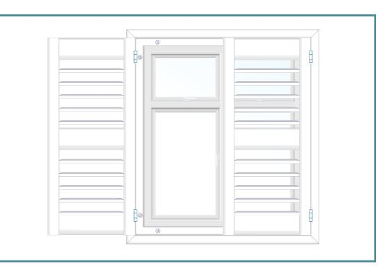
Check that your panels open and close easily. As they can be heavy, it's normal if you need to lift the edge of the panel and nudge it on.
