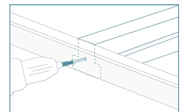
If you have T posts, screw them onto your shutter frame using your cordless drill and the long black screws in your custom kit. There are pre drilled holes on your shutter frame, to show where you'll attach the T posts. The top of your T post will be labelled t, and the bottom b.
