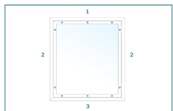
Drill in your side screws next, and then your bottom screws. You can check your shutter frame is even across the top by using a spirit level.
