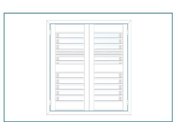
Check for a thin, even gap between each side of your shutter frame and your shutter panels.
