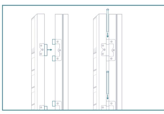
Remove any black bands from your hinge pins before you start. Pick up your left panel and hold into position. The brackets should line up on the left side of your shutter frame and your panel. Take a hinge pin and drop it through the bracket, from the top. Repeat for each panel.
